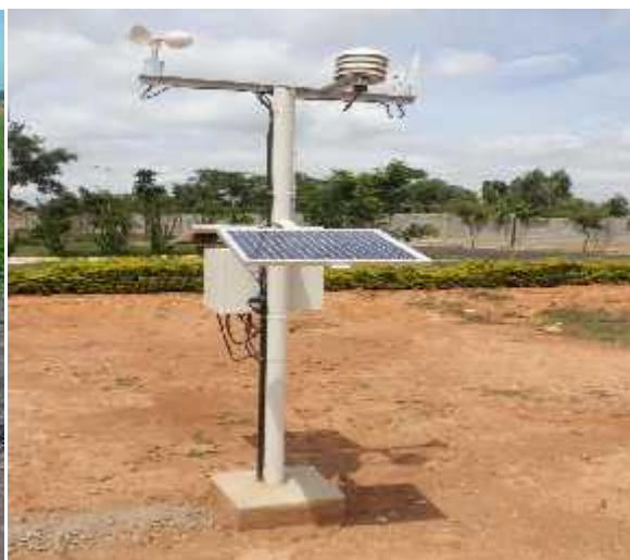
Telemetric Weather Station
